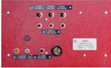
Metron alarm panels have been designed to provide reliable audible and visual alarms for electric and diesel fire pump controllers in accordance with NFPA 20. This requires that visual and audible alarms powered by a reliable source, not exceeding 125 volts, be located at a point of constant attendance when the pump room is not constantly attended.
